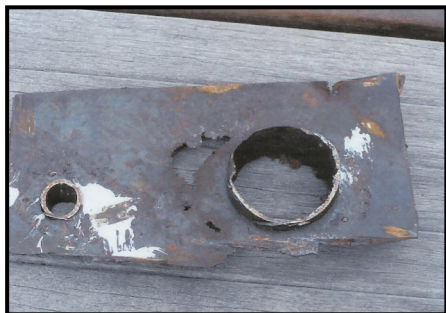
Tanks rotted through around filler inlet
