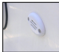
Port fairing with Eberspacher air intake
